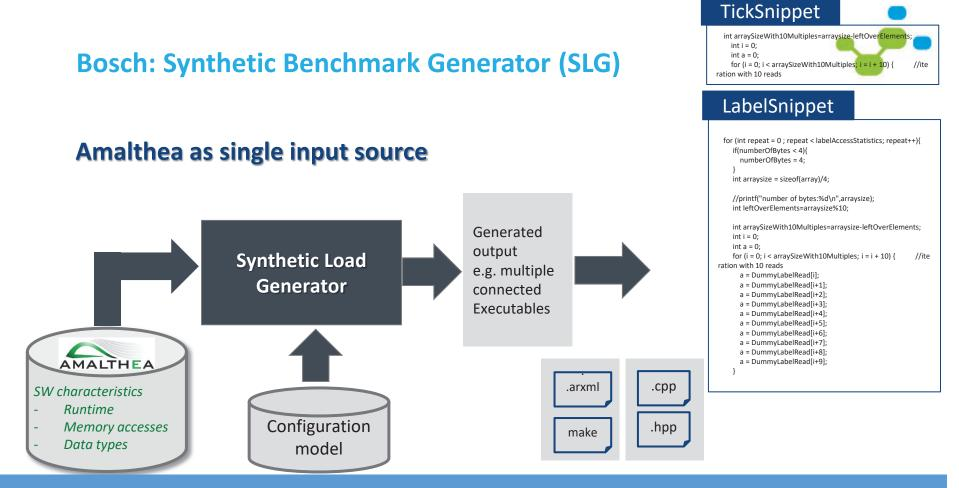
Generating Executables which are directly deployable on the ECU
