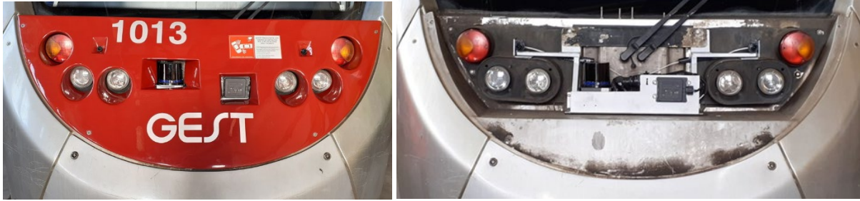
Figure 2-4: Sensors installation on board of streetcar 1013. The radar, LiDAR, and stereo camera are visible in the left figure where the tram nose skin is shown and in the right picture where it was removed and shows the relevant brackets.
